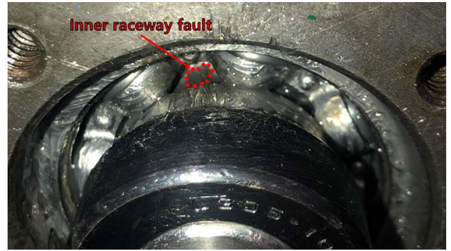
FIGURE 4. Faulted ball bearing of centrifugal pump in Ajou University using a drill, and the fault is located on the inner raceway.
