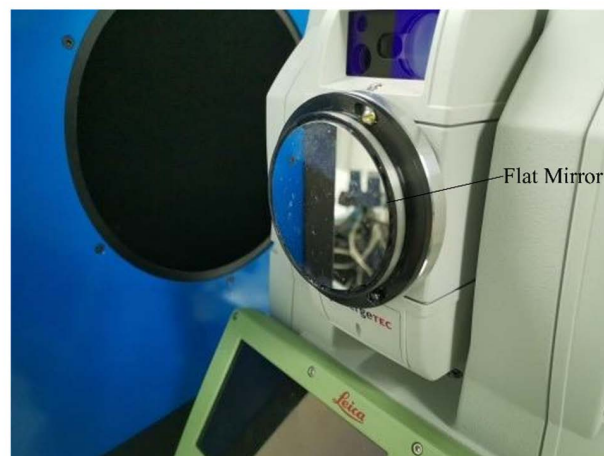
FIGURE 11. Flat mirror is fixed on the Leica MS60 Electronic Total Station.
