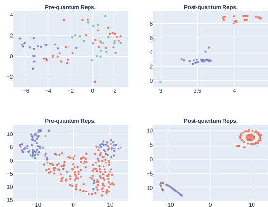
FIGURE 14. Analysis on representation learning pre- and post-quantum embeddings using T-SNE: (Top) Wine dataset, (Bottom) Breast Cancer dataset. The T-SNE features from pre-ansatz representations is hard to be separated using linear classifier, while those features from post-representations can be well-separated using the same classifiers.
