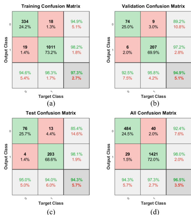
FIGURE 8. CYP3A4 prediction model evaluation confusion matrix. (a). Training confusion matrix. (b). Validation confusion matrix. (c). Test confusion matrix. (d). All confusion matrix.
