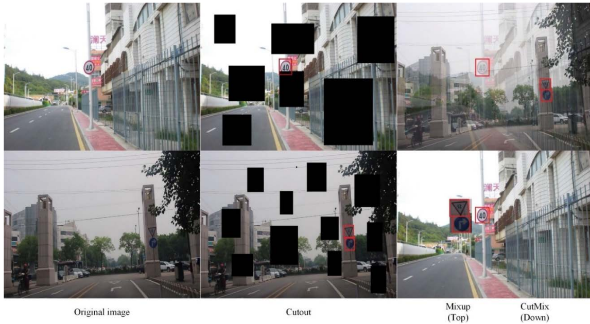
FIGURE 6. Data augmentation for traffic object. On the basis of commonly used data augmentation, Cutout, Mixup and CutMix were used to increase variety of image data.
