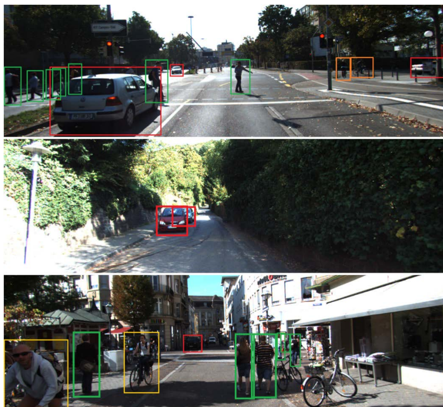
FIGURE 9. Detection Results on KITTI dataset. The above figure shows the proposed algorithm accurately detecting objects in a traffic scene on the KITTI object detection dataset.
