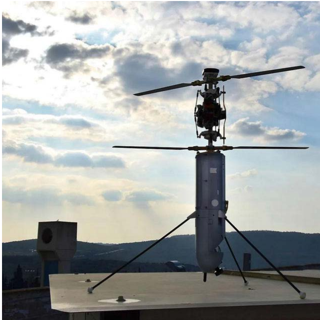
FIGURE 3. The Israel “FireFly” coaxial rotorcraft.
