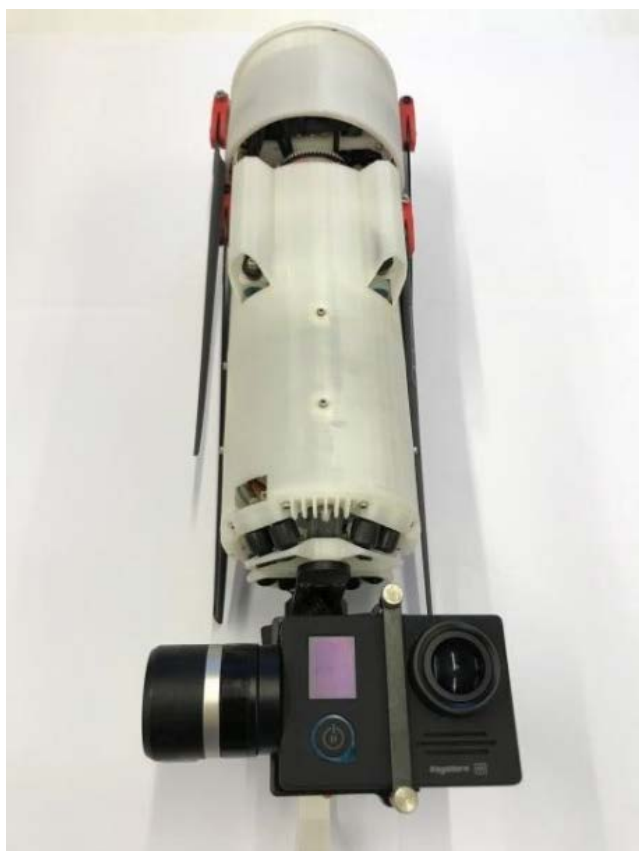
FIGURE 6. The open source “TDrone” coaxial rotorcraft.
