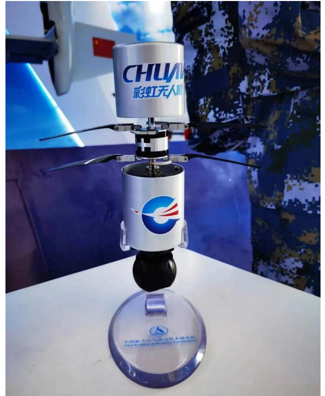
FIGURE 4. The China “CH-817” coaxial rotorcraft.
