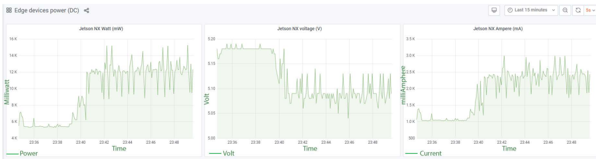
FIGURE 13. Status monitoring of the power consumption of Jetson Nano while running the SSD object detection methods.
