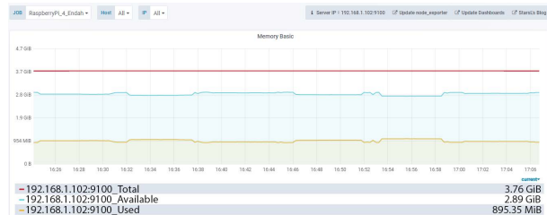
FIGURE 16. Resource changes of memory when running the three unoptimized models with FP16 and FP32.
