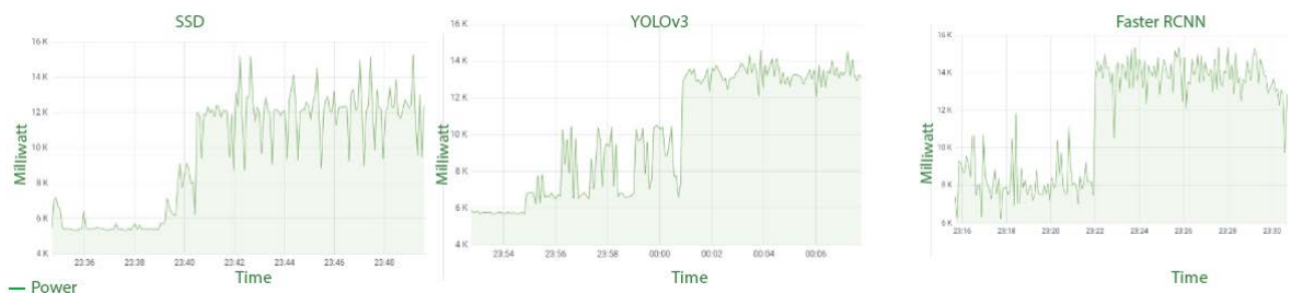
FIGURE 14. Comparison of power consumption using Jetson Nano for different object detection methods: (a) SSD, (b) YOLO, and (c) Faster R-CNN.
