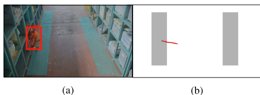
FIGURE 21. Examples of safety zone violations for fixed areas using CCTV images: (a) Images, (b) Trajectories in the top-view plane.
