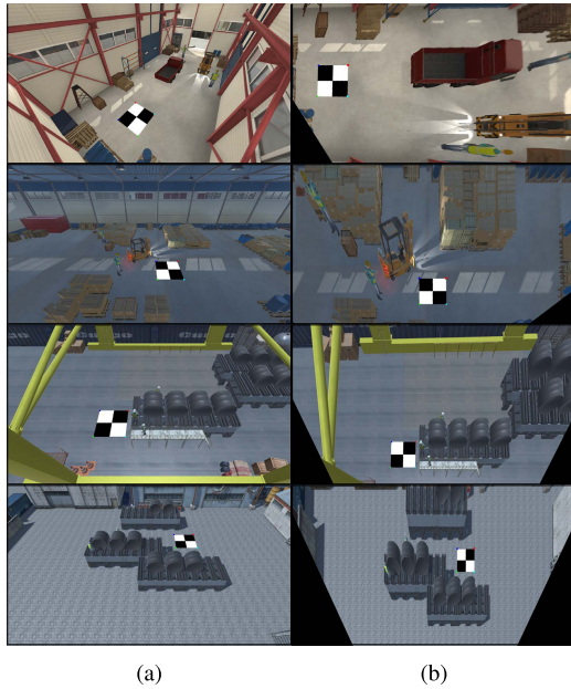
FIGURE 4. Examples of perspective transforms using Unity 3D simulation: (a) Images from virtual cameras at vantage points; (b) Top-view plane images.
