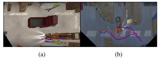
FIGURE 9. Examples of trajectory estimation with Unity 3D images. Blue: estimated trajectory, Red: ground truth.
