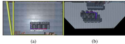
FIGURE 14. Examples of trajectory estimation using Unity images. Blue: estimated trajectory, Red: ground truth.
