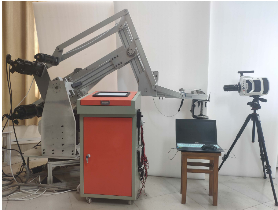
FIGURE 12. Experimental test system for the residual vibration of the CM robot.
