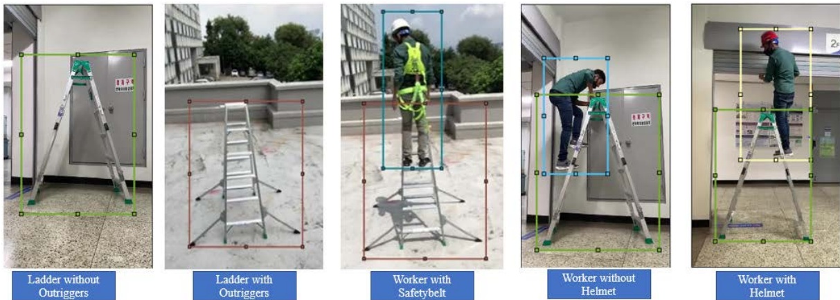
FIGURE 5. Dataset labeling for the SSD-based object detector.
