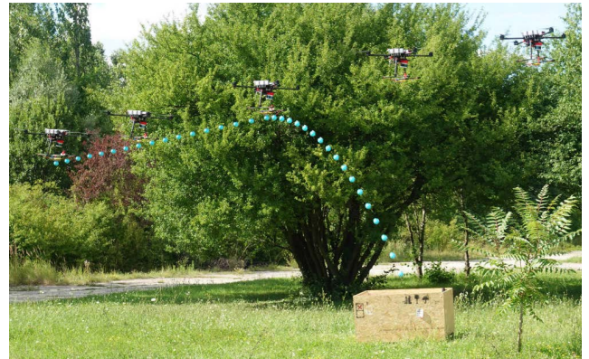
FIGURE 1. An illustration of an experiment performed outdoors. The UAV carries the ball to the release point and executes the stopping motion afterwards. After the release instance, the free-fall parabolic trajectory can be observed.
