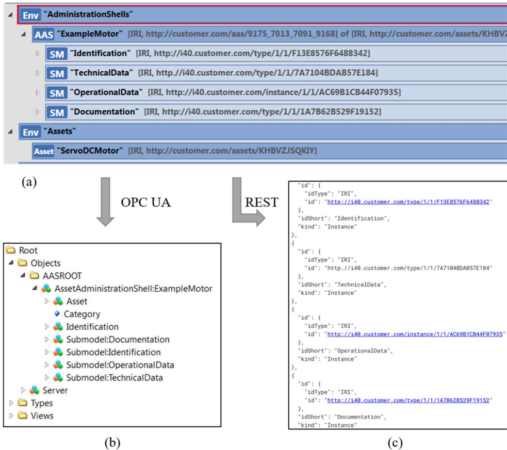
FIGURE 4. An AASX package explorer and the AASX information accessed via OPC UA and REST. (a) AAS information shown in the AASX package explorer. (b) AAS information shown in UaExpert. (c) AAS information shown in JSON.
