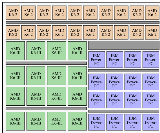
FIGURE 2. Floorplan of the many-core platform used in the experiments. Processing cores are denoted by squares where the core types are reflected by color and noted on the cores. Communication resources and shared memories are contained in the gray regions.
