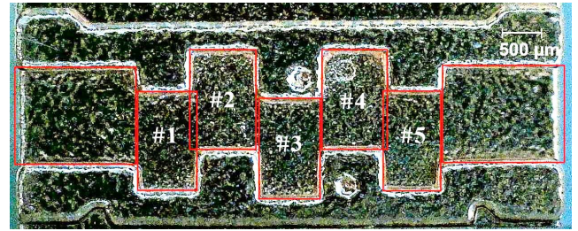
FIGURE 20. Microphotograph of the bottom part of our non-pre-distorted G-band 5 th order chained-function filter (after plating). The red rectangles represent the recorded boundary dimensions.
