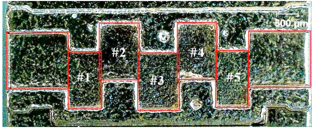
FIGURE 22. Microphotograph of the bottom part of our fully pre-distorted G-band 5 th order Chebyshev filter (after plating). The red rectangles represent the recorded boundary dimensions.
