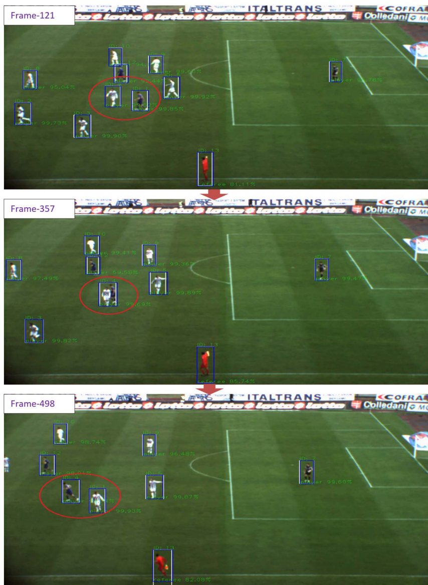
FIGURE 9. Tracking results in the case of identity switching Using YOLOv4 + Deep-SORT, which can be seen in the red circle (Frame-121 to Frame-498).
