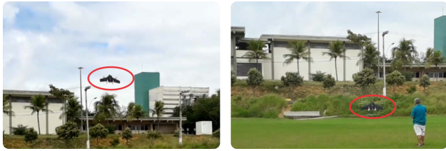
FIGURE 28. Transition from airplane (fuelled) to hovering (multirotor) mode (left picture), just before landing (right picture).
