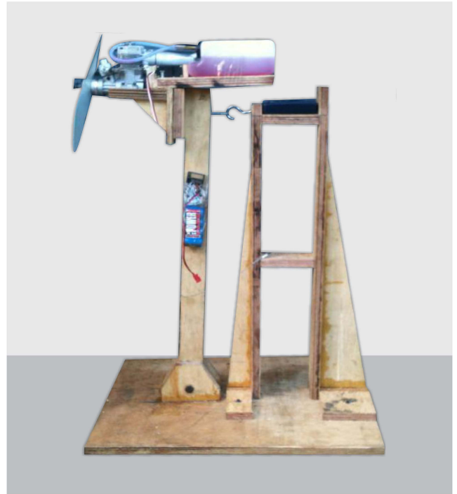
FIGURE 29. Bench developed for testing flight time endurance.
