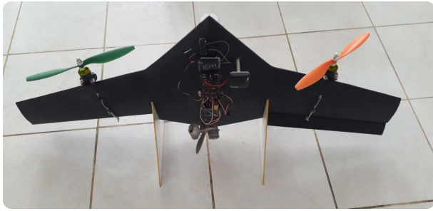
FIGURE 23. Complete assembly of the main UAV structure painted with a vinyl coating.
