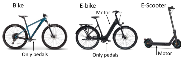
FIGURE 9. From left to right: bike, e-bike and e-scooter. The e-bike has a motor that adds additional push while the biker is pedalling. The e-scooter has a motor and it does not require the biker to pedal.
