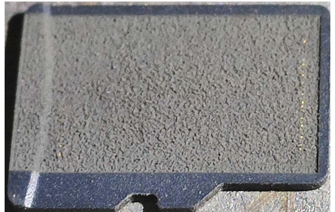
FIGURE 27. Example of a micro-SD card after laser preparation.
