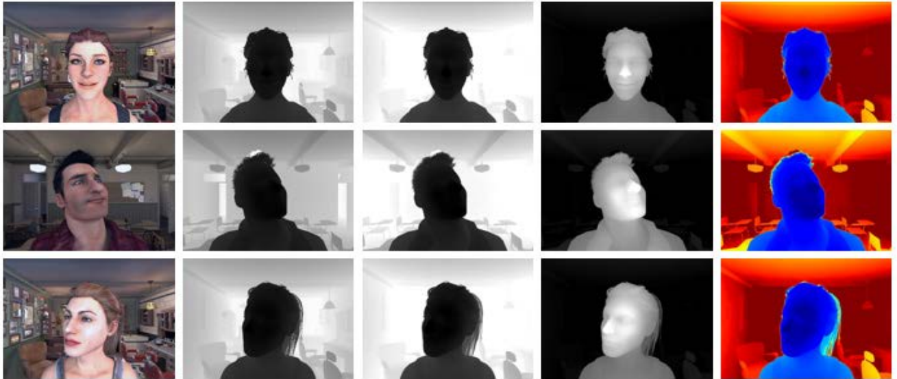
FIGURE 4. Qualitative results in a sample of the synthetic human facial test dataset that was not used for training or validation. Input RGB images, ground truth images, predicted depth images, predicted depth images (Greys), and predicted depth images are shown from left to right.
