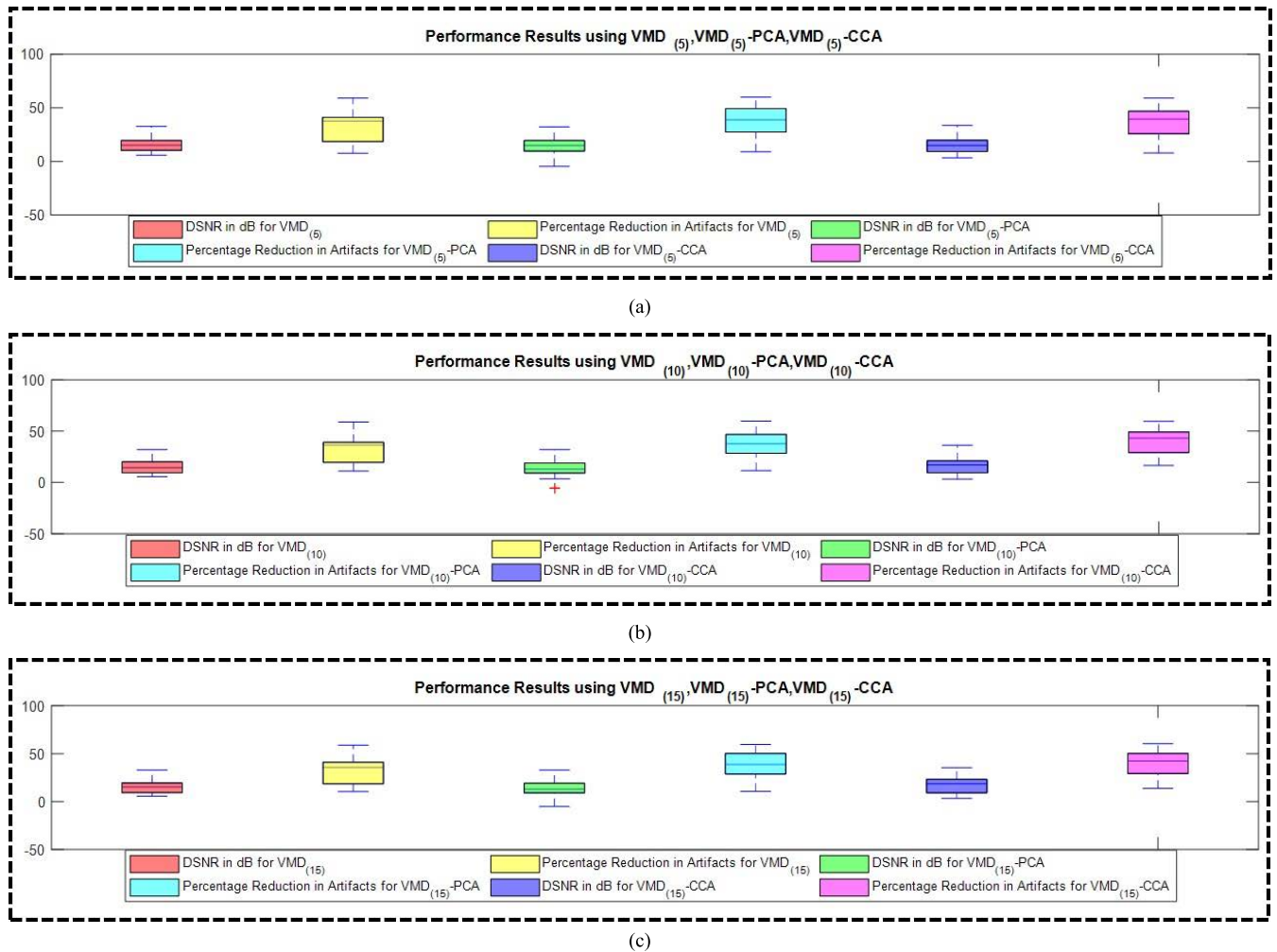
FIGURE 14. Box and whisker plot of performance parameters using (a) VMD_{(5)} , VMD_{(5)} -PCA, and VMD_{(5)} -CCA, (b) VMD_{(10)} , VMD_{(10)} -PCA, and VMD_{(10)} -CCA, and (c) VMD_{(15)} , VMD_{(15)} -PCA, and VMD_{(15)} -CCA for 15 denoised fNIRS signals.
