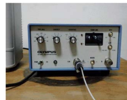
FIGURE 1. (a) PZT ultrasonic sensing chips fabrication processes.; (b)The fabricated sample; (c) The utilized pulser/receiver; (d) The utilized digital oscilloscope for recording the ultrasonic signals during the experiments.
