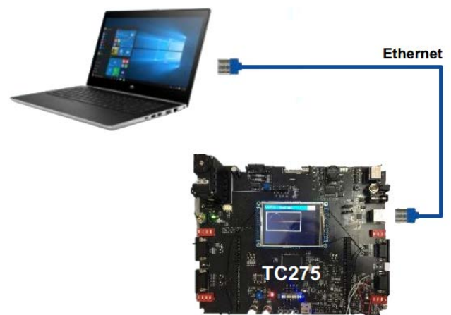
FIGURE 13. Ethernet interface structure of TC275.
