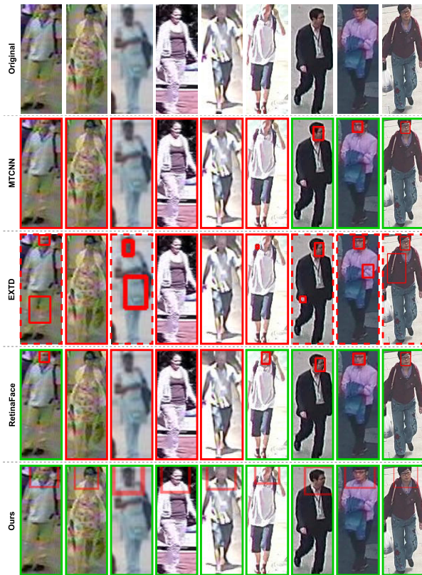
FIGURE 4. Comparison of the head ROI detection results between MTCNN, EXTD, RetinaFace, and our approach, in images with varying quality, head pose and blurriness. Green boxes denote cases where the method accurately locates the face, and red boxes denote the opposite. Dotted red boxes refer to cases where the model over-predicted the number of existent faces. All images are resized to the same resolution for visualization purposes.
