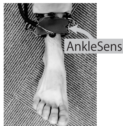
FIGURE 5. A snapshot of the device. We have placed AnkleSens between the upper part of the ankle and the shin.
