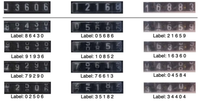
FIGURE 6. Counter images produced with the proposed generative augmentation. Above the line are the original images. Under the line are the generated images and their automatically annotated labels.
