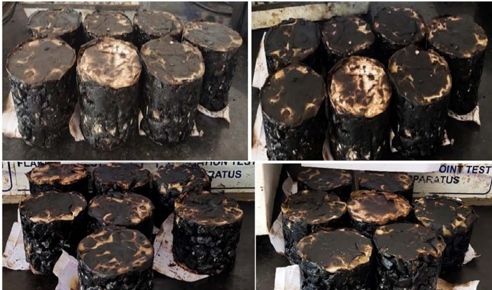
FIGURE 4. Glass fiber reinforced asphalt specimens.
