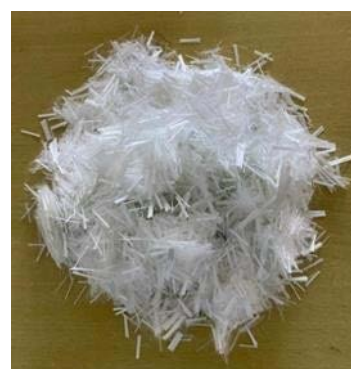
FIGURE 3. Glass fiber utilized in this study.
