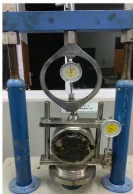
FIGURE 5. Marshall steadiness apparatus used in testing.
