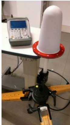
FIGURE 5. Equipment for spectrum evaluation: Rhode & Schwartz FSH6 spectrum analyzer and receiving antenna on tripod ETS-LINDGREN, Mod. 3182.
