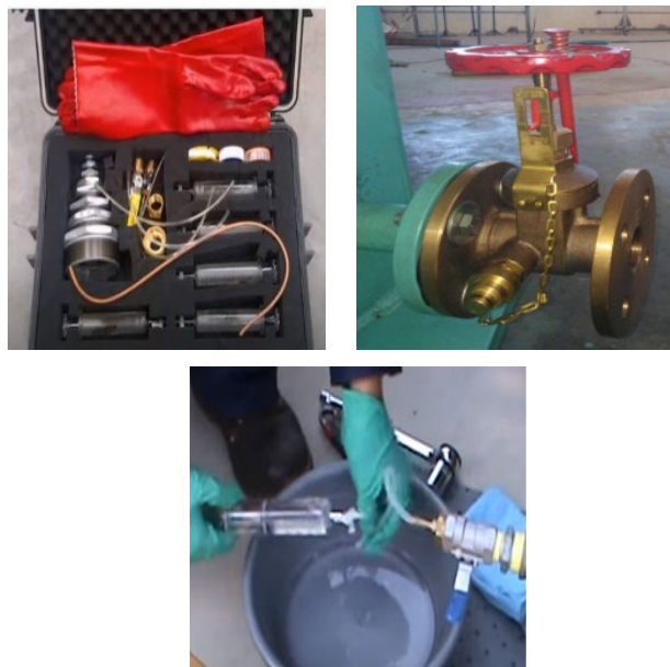
FIGURE 10. Dissolved gas analysis sampling process and used tools.
