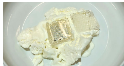
FIGURE 15. Photograph of the prototypes on ice cream to observe the change in reflection intensity over time.
