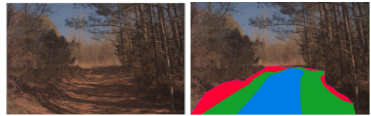
FIGURE 1. Example of traversability assessment in camera images. Left: original image, right: traversability labels overlaid onto the image where red, green and blue colors correspond the traversable areas by off-road, pickup, and sedan type vehicles. In this specific example, due to the absence of other irregularities on the road, the only difference between the road parts that could be traversed by each vehicle type is in-terms of the extent on two sides of the road it can travel.
