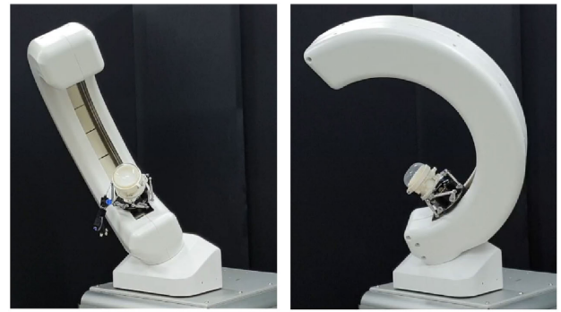
FIGURE 12. Feasibility test of the revolute joint in the brain stimulation robot.
