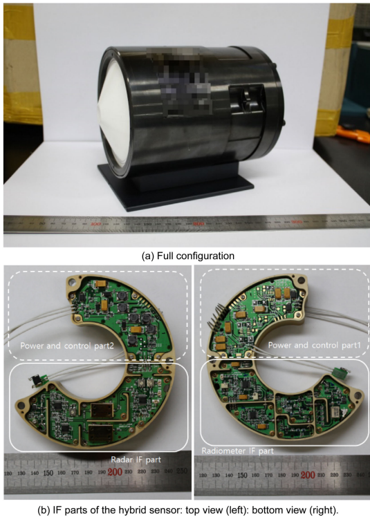
FIGURE 11. The fabricated hybrid sensor based on miniaturized FMCW radar and TPR.
