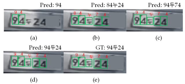
FIGURE 13. SR (x4) and character recognition results of plate images with (a) DBPN+TesseractOCR, (b) super-resolved recognition, (c) DBPN + OpenALPR, (d) collaborative learning result, and (e) HR image (80 x 60), respectively. "GT" represents ground-truth and "Pred" represents prediction results.
