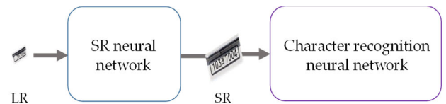
FIGURE 1. An overall diagram of the proposed collaborative trainable neural network.
