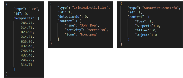
FIGURE 6. An example of 3 Information Elements. The one on the left corresponds to a 'Detection' component type ('Foe') the middle one to an 'Annotation' component type ('CriminalActivities'), and the right one to a 'General' component type ('SummativeSceneInfo').
