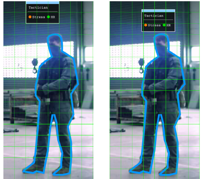
FIGURE 8. Positioning of an annotation in terms of grid tiles (left) and in terms of pixels (right). The sampling rate is 60px.
