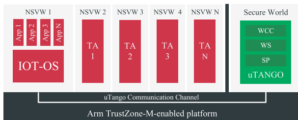
(b) uTango TEE architecture with a novel multi-world model. Compared to a), solely uTango sits on the secure world, while everything else (including trusted applications) is assigned and isolated in an NSVW.
