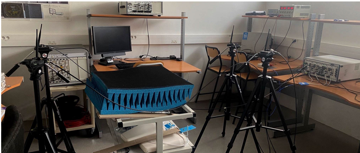
FIGURE 11. Experimental setup of a 2 × 2 SM system with realistic propagation environment.
