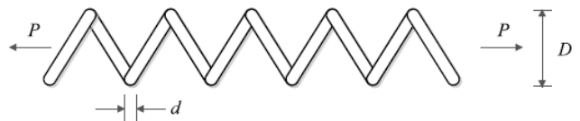
FIGURE 12. Schematic view of tension/compression spring problem.
