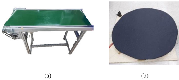
FIGURE 12. Two laboratory-made object moving platforms: (a) a conveyor and (b) a circular rotating platform.
