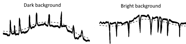
FIGURE 4. One dimensional representation of a grayscale image and the desired threshold (dotted line) for fracture segmentation considering either with a dark or bright background. Adapted from [46].
