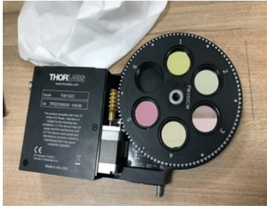
FIGURE 3. A closer look at the spectral filters mounted on a motorized filter wheel.
