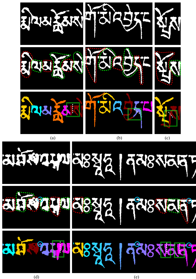
FIGURE 16. Examples of the limitations of character detection and segmentation algorithm. (a) The touching point is located in the HC. (b) and (c) The touching point is located in the concave stroke. (d) The handwriting is at will or the original image is of low quality and the character stroke features are not obvious. (e) Complex touching and breaking among strokes of multiple characters.
