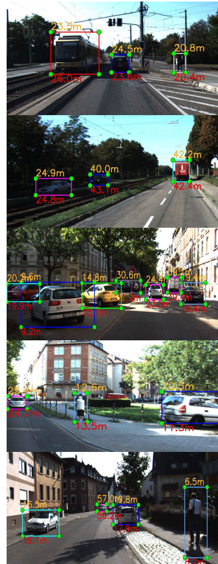
FIGURE 4. Results on KITTI [10]. The predicted depth (yellow) is on the upper side of the box and the ground truth depth (red) is on the lower side of the box.
