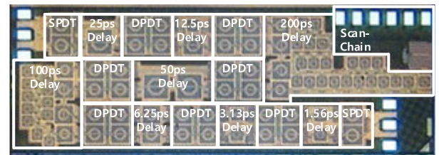
FIGURE 12. Chip-photograph of the fabricated 5-11 GHz 8-bit true-time delay (TTD) in 65-nm CMOS technology.
