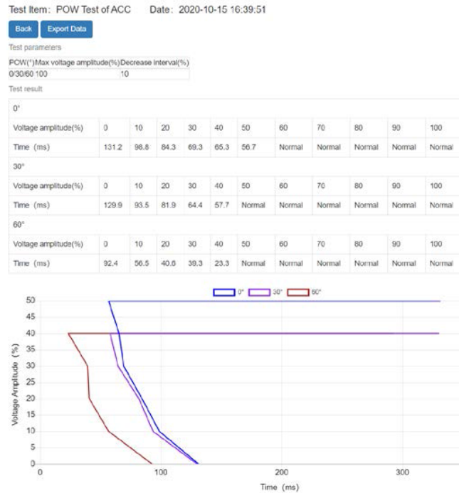
FIGURE 19. Diagram of the test result of ACC in the user interface of the automatic test system.
