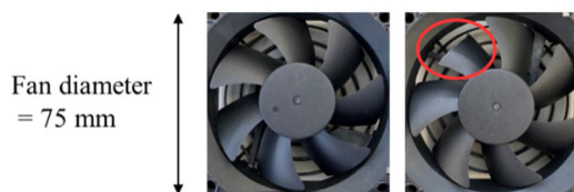
FIGURE 2. Normal propeller (left) and a failed propeller (right).
