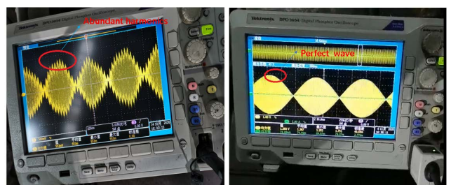
FIGURE 17. Waveforms before and after the interference of the rotary transformer signal.
