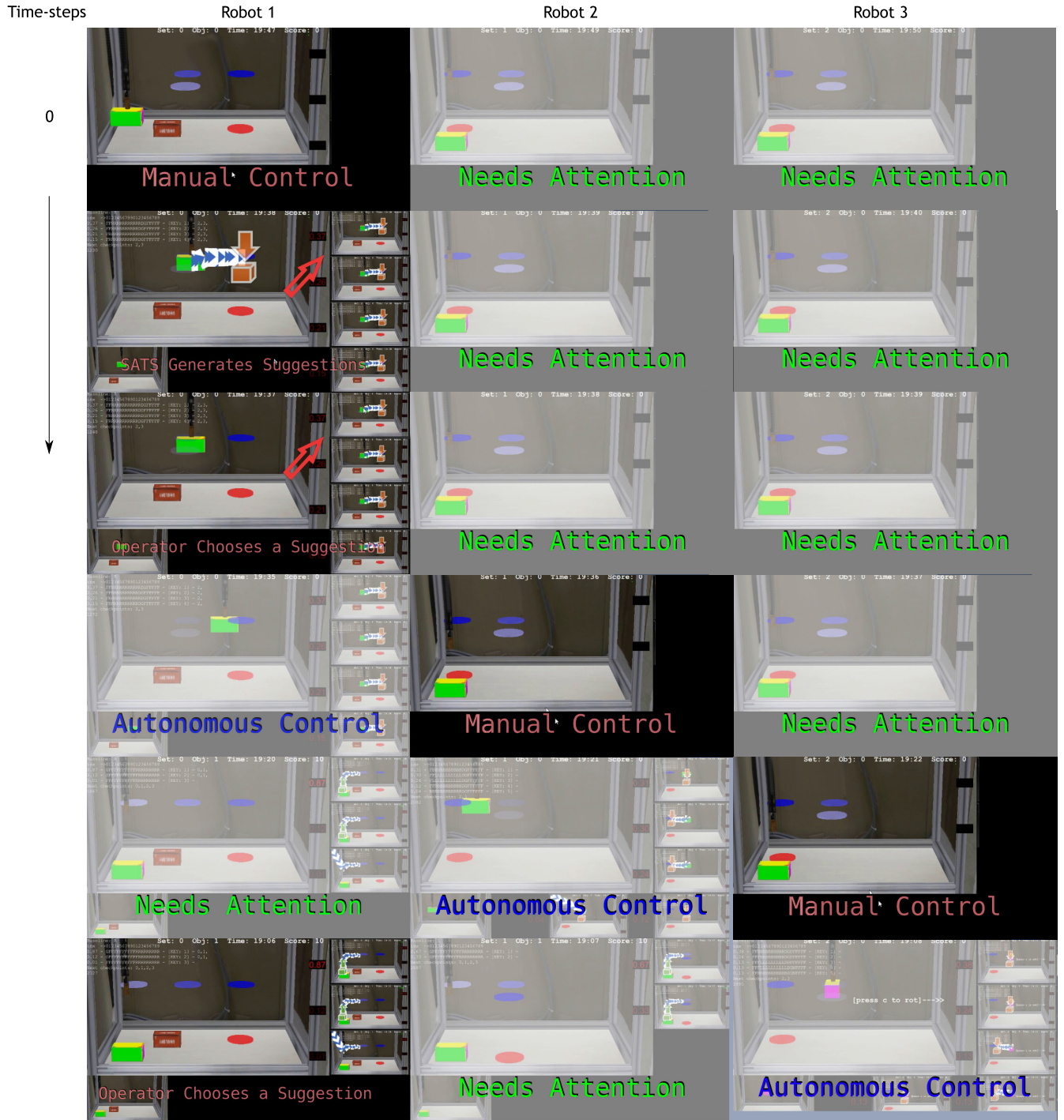
FIGURE 10. Visualization of simultaneous multi-robot control using the proposed system. Each column shows snapshots from a different environment. Each row demonstrates a step while the operator uses SATS (Refer to supplementary material for more results).
