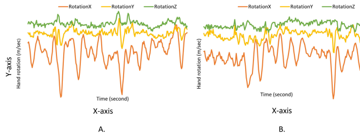
FIGURE 6. Data correction: A. shows original average skeletal hand video frames, and B. represents smoothed and corrected frames information using weighted linear regression.
