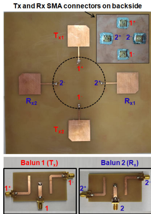
FIGURE 6. The validation models of antenna and two slot-fed baluns for balanced T_x and R_x feeding of two pairs of co-RHCP patches.
