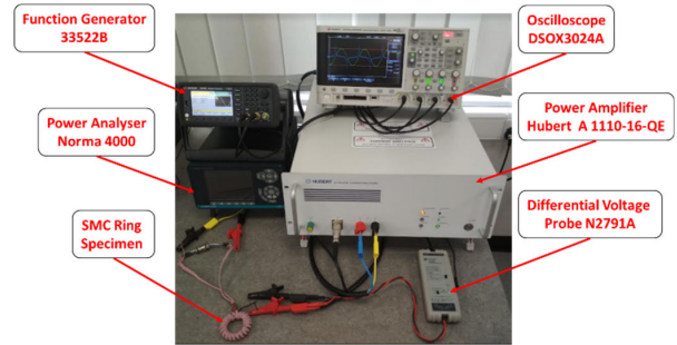
FIGURE 7. Iron loss measurement setup.
